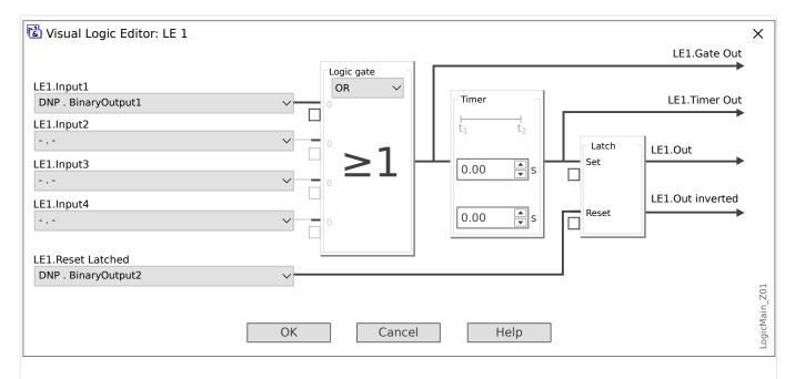
Fig. 37: Setting example from Smart view, to make a steady state signal from a DNP output signal.
