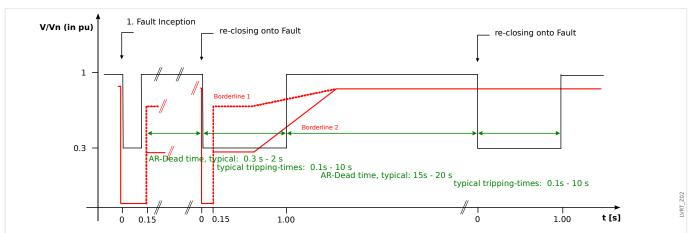
Fig. 58: Run of voltage curve during an unsuccessful two-shot auto reclosure; source: VDE-AR-N 4110/4120.
