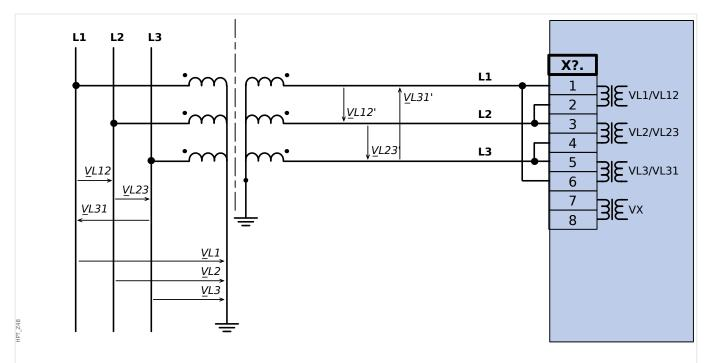
Fig. 19: Three-phase voltage measurement - wiring of the measurement inputs: "delta-connection"
