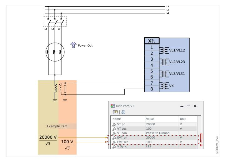
After the voltage inputs have been connected correctly the residual voltage is measured with the following setting:
