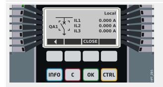
The Softkey "▶" (Enter) takes you to an enhanced single line (after you have entered the password for access level "Control-Lv1"). The switchgear device is highlighted by small markers (and in case of several implemented switchgear devices, the Softkey "Select" is visible, which allows you to select another one).
