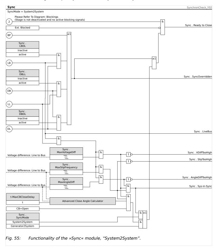
Setting: [Protection Para / Set x / Intercon-Prot / Sync / Mode / Times] \*SyncMode\* = "System2System"
