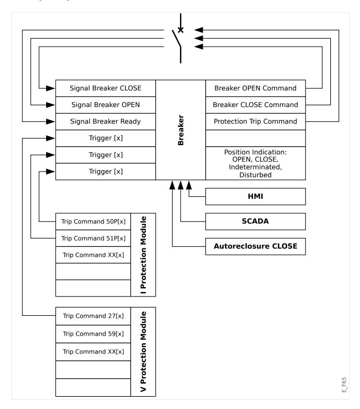
In the menu [Control / Qxx / Trip Manager] (where "Qxx" corresponds to the designation of the switchgear, as it is defined in the single-line diagram), there are setting parameters »Off Cmd n«, to which you can assign the protection trip commands. In this so-called Trip Manger, all these assigned protection trip commands are combined by an "OR" logic, which then cause a switchgear trip command to be issued.
