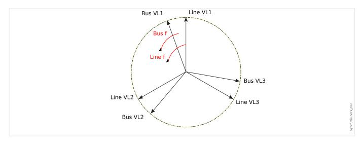
If the generator frequency fBus is not equal to the mains frequency fLine, it results in a slip frequency  $\Delta F = |fBus - fLine|$  between the two system frequencies.
