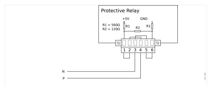
Wiring example, Device at the end of the bus. (Setting wire jumpers to activate the integrated Terminal Resistor.) Fig. 30:
