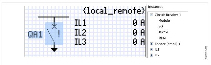
Fig. 64: Control Page Example, with the "Circuit Breaker" being highlighted.
