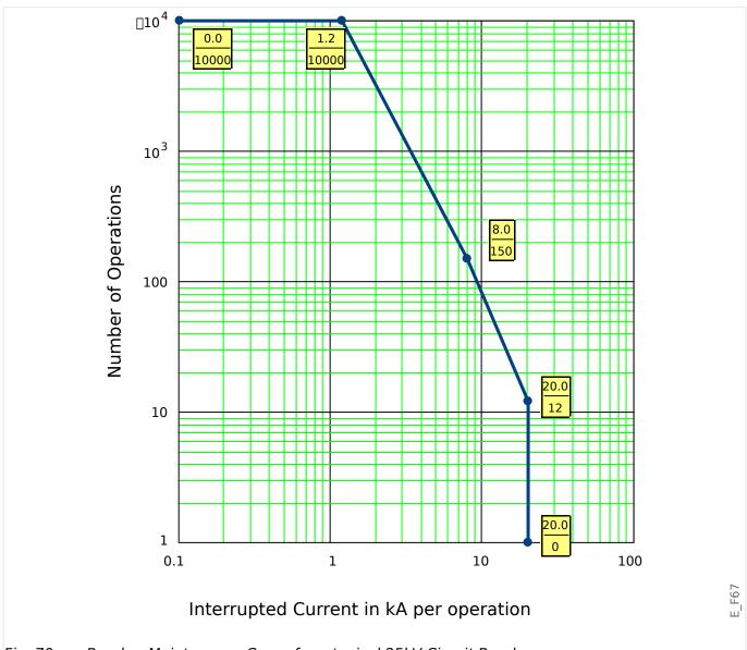
Fig. 70: Breaker Maintenance Curve for a typical 25kV Circuit Breaker
