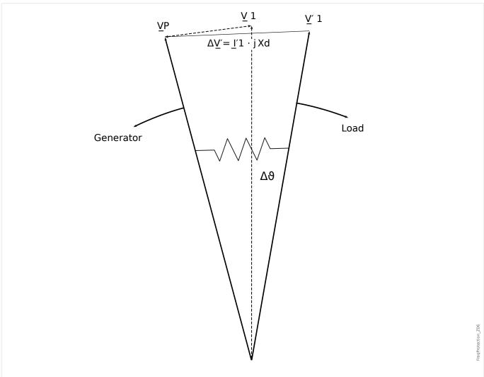
Fig. 49: Voltage vectors at mains failure.
