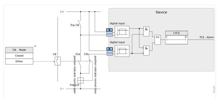
Fig. 62: Connection example: Trip circuit supervision with two CB auxiliary contacts »Aux ON« (52a) and »Aux OFF« (52b).
