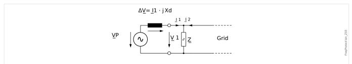
Fig. 46: Equivalent circuit at synchronous generator in parallel with the mains.
