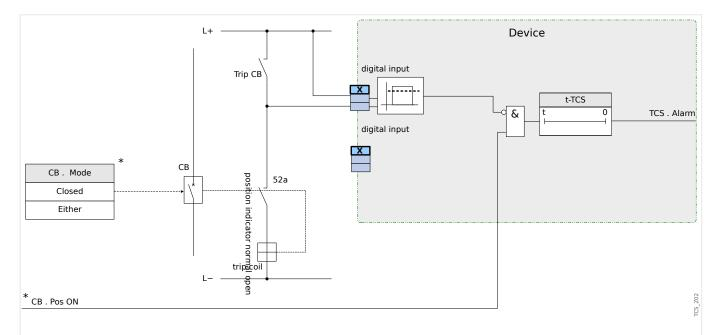
Connection example: Trip circuit supervision with only one CB auxiliary contact »Aux Fig. 63: ON« (52a).
