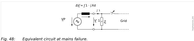
Tig. 46. Equivalent circuit at mains failule.
