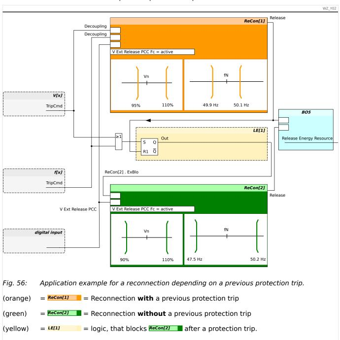
According to TR3, the release ranges (orange) that are used after a protection trip have to be smaller than the release ranges (green) without a previous trip. The example above configures the first reconnection instance, »ReCon[1]«, for the small (orange) ranges, and the decoupling functions are assigned to this instance.
