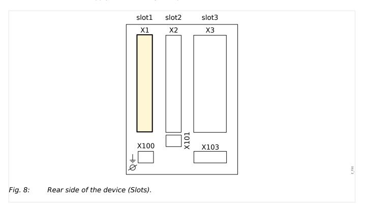
The type of power supply card and the number of digital inputs on it used in this slot is dependent on the ordered device type. The different variants have a different scope of functions.
