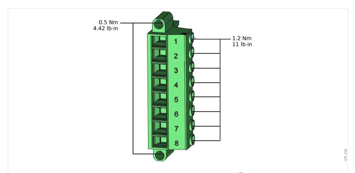
Fig. 81: Voltage measurement terminals of measuring card "TU" (╚⇒ "2.5.1 TU - Voltage Measuring Inputs").
