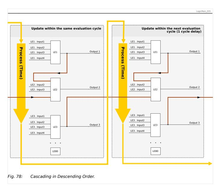
In the example shown in  $\sqsubseteq$  Fig. 78 above, "Logic Equation **2**" uses the output states of two other equations, "Logic Equation **1**" and "Logic Equation **3**". The result of "Logic Equation **1**" is used in ascending order and has therefore been evaluated within the same process cycle. The result of "Logic Equation **3**" is used in descending order and has therefore been evaluated in the previous process cycle.
