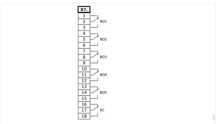
Fig. 12: RO-5 - Terminal Marking
