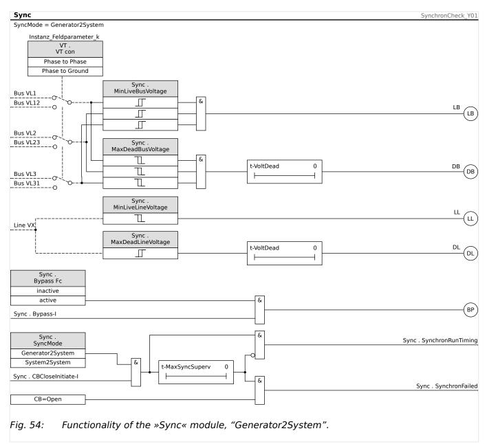
Setting: [Protection Para / Set x / Intercon-Prot / Sync / Mode / Times] »SyncMode« = "Generator2System"
