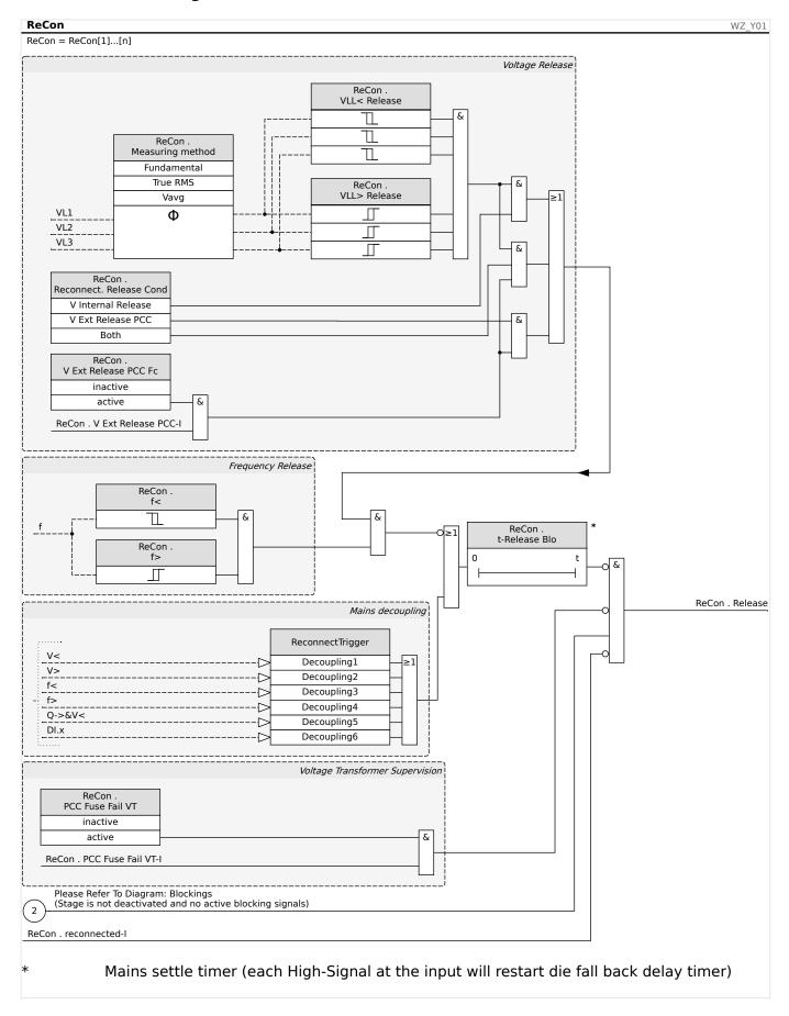
The tile "Mains decoupling" in the diagram shows the available decoupling signals that can be assigned as trigger signals. The reconnection checks can be triggered from up to 6 decoupling functions, or via Digital Inputs, logic equations or SCADA connection.
