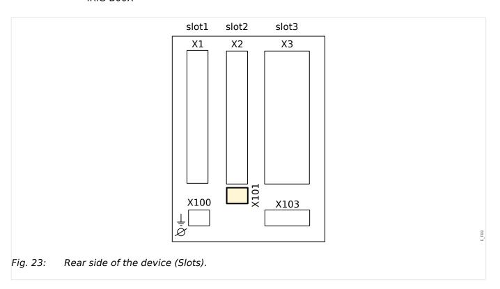
Depending on the ordered device type, this slot can be equipped with an IRIG-B interface.
