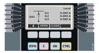
Fig. 66: Control Page Example, with the "Circuit Breaker" in faulty (or implausible) position.
