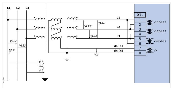
Fig. 20: Three-phase voltage measurement - wiring of the measurement inputs: "delta-connection"Measurement of the residual voltage VG via auxilliary windings (e-n) "broken delta"
