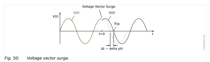
As shown in the voltage/time diagram the instantaneous value of the voltage jumps to another value and the phase position changes. This is called phase or vector surge.
