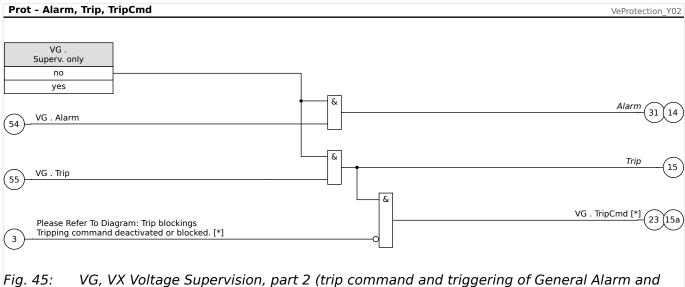
The trip command and its blocking exist only for the setting »Superv. only « = "no"
