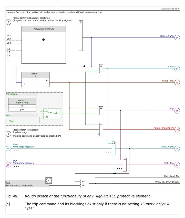
This diagram shows the basic idea behind a protective element. (Nevertheless, keep in mind that device-specific or protection-specific deviations are possible: Some devices do not feature voltage measurement, other do not feature current measurement, for some protection elements other timers and/or phase-specific algorithms are required, etc. So, for the exact functionality of a protection module please consult the respective chapter.)
