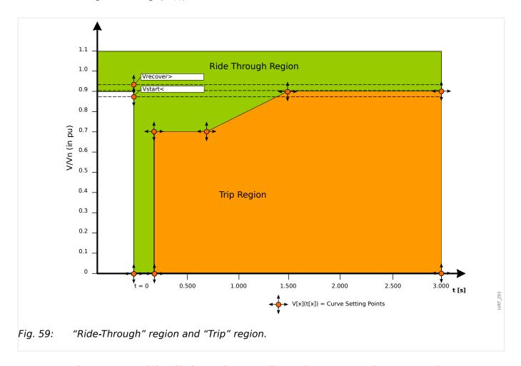
The »LVRT« module will change into standby again as soon as the system voltage recovers: That means, the voltage has risen above the preset recover voltage »Vrecover>«.
