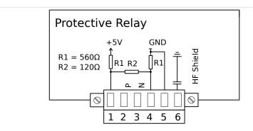
Fig. 28: Electro-mechanical assignment
