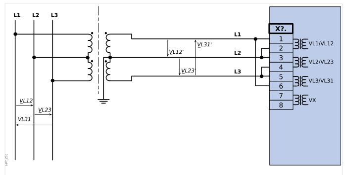
Fig. 21: Two-phase voltage measurement - wiring of the measuring inputs: "Open Delta"
