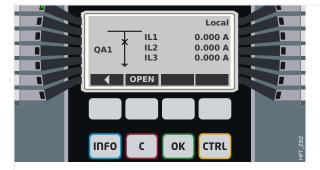
Fig. 65: Control Page Example, with the "Circuit Breaker" in closed position.
