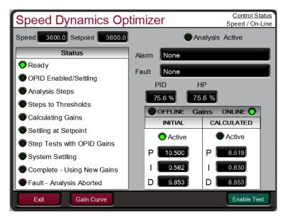
Figure 4-35. Overview of the Automated PID Optimizer Routine
