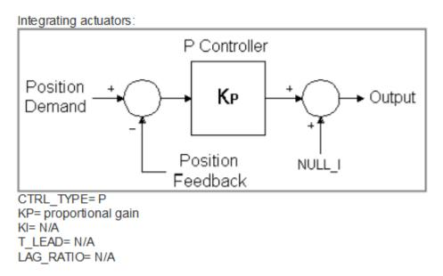
Figure 1-11. Integrating actuator using P controller
