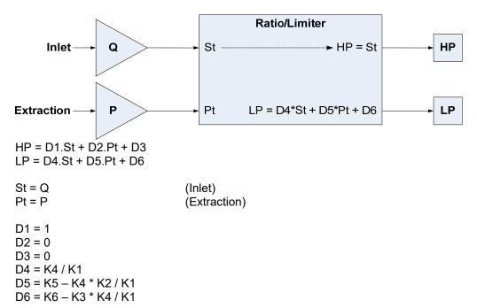
The inlet pressure is determined by HP demand only, without any effect of LP. (St = HP)
