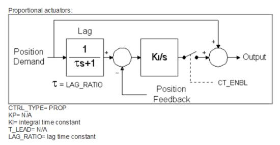
Figure 1-10. Proportional actuator with command trim
