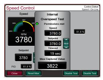
Figure 4-29. Internal (Control) Overspeed Test
