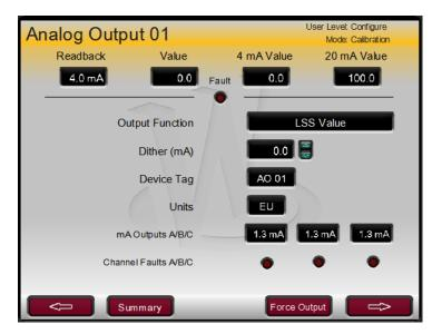
Figure 3-6. Analog Output Channel Calibration Mode
