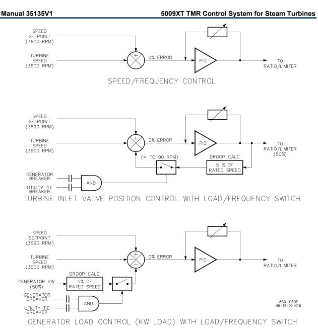
Figure 2-8. Speed PID Control Modes
