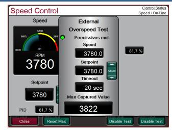
Figure 4-30. External Overspeed Test
