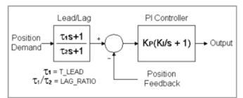
CTRL\_TYPE=PI\_LEADLAG KP= proportional gain KI= integral gain T\_LEAD= lead time constant LAG\_RATIO= lead/lag ratio
