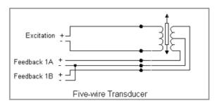
The "+" and "-" designations shown here are arbitrary. The (-) side of the feedbacks 1A and 1B should be tied to the output center tap as shown.
