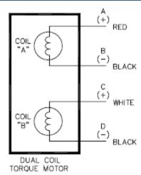
Figure 1-8. Dual coil torque motor
