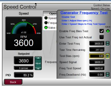
The test allows two forms of simulated test values. By default, a Test Bias (rpm) can be added (or subtracted if negative) to the current frequency value. For example, if turbine speed is 3600RPM, to simulate an increase in grid frequency of 0.1%, a bias signal of 3.6RPM can be added. **Note:** below, the PID amount decreased in response to the increase in grid frequency.
