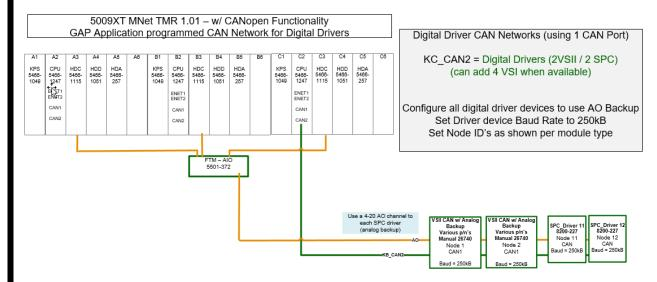
Figure 1-17a. CAN links to Distributed Drivers
