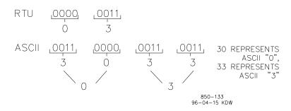
Figure 6-1. ASCII/RTU Representation of 3
