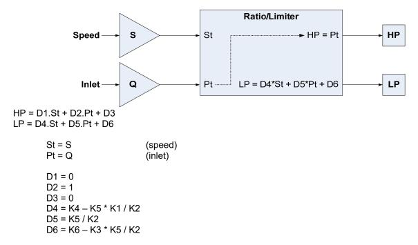
The inlet pressure is determined by HP demand only, without any effect of LP. (Pt = HP)
