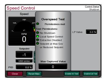
Figure 4-28. Overspeed Test Permissives
