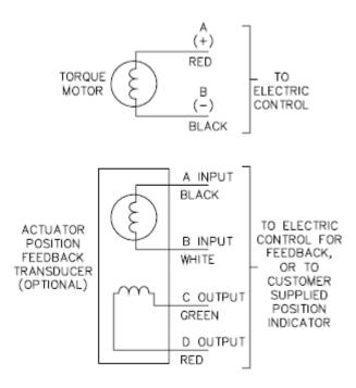
Figure 1-7. Single torque motor with feedback
