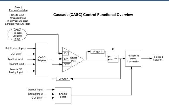
Figure 2-13. Cascade Functional Diagram
