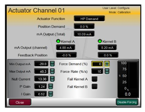
Figure 3-16. CALMODE - Forcing mode enabled for integrating valve
