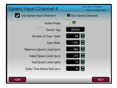
Figure 2-1. Speed Probe Zero Speed Detect
