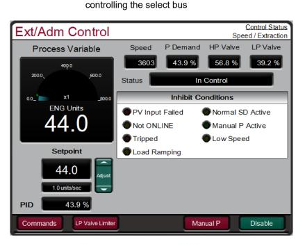
Figure 2-21. Extraction/Admission Control Panel
