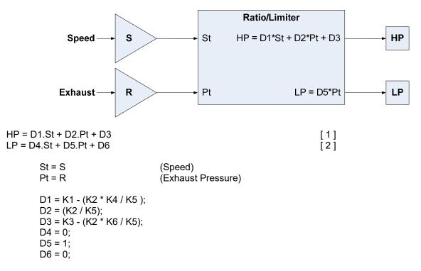
This mode is used when the two controlled parameters during normal operation are turbine speed/load and exhaust pressure (or flow).
