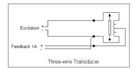
Figure 1-15. Three wire feedback device
