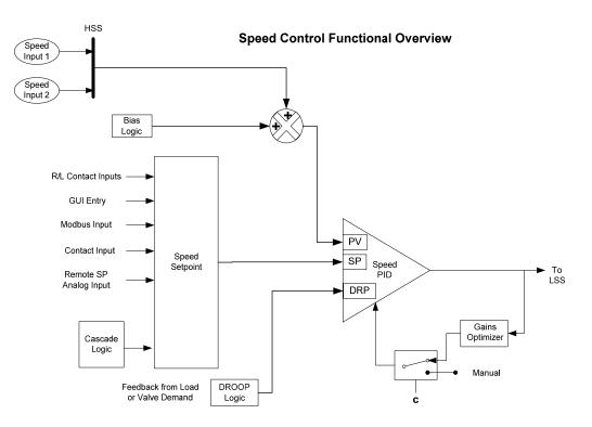
Figure 2-7. Speed Control Functional Diagram
