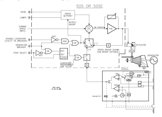
Figure 2-11. Load Sharing Logic
