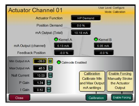
Figure 3-9. CALMODE access to Calibration and Forcing (Stroking)
