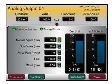
Figure 3-7. Analog Channel Forcing Mode
